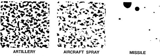
Figure 1-2. Moderate liquid contamination on M9 paper (1 gram/square meter).
